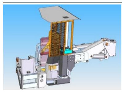
protecting the operator from rib rolls regardless of the canopy height.
