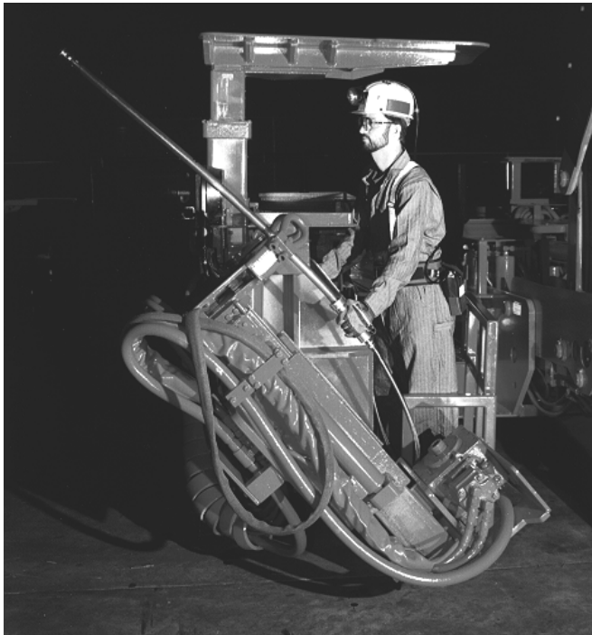
Resin Inserter used on mast feed Fletcher roof bolter.
