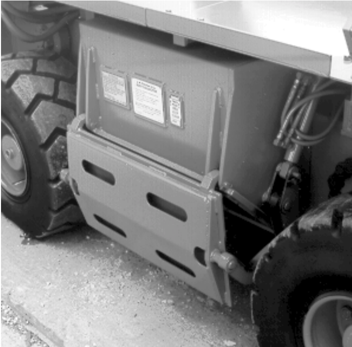
Auto-Dump Dust Tank
