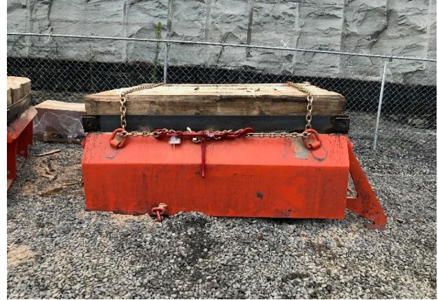
Figure 4. MRS Extension, (OEM and mine supplied wood layer), located adjacent to Rockhouse Eagle Face-up and Coal Outcrop
