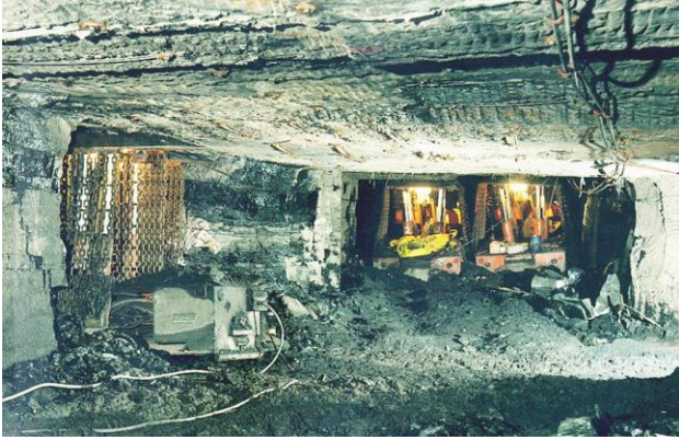
Figure 1. Mobile Roof Supports underground deployed in pairs.
