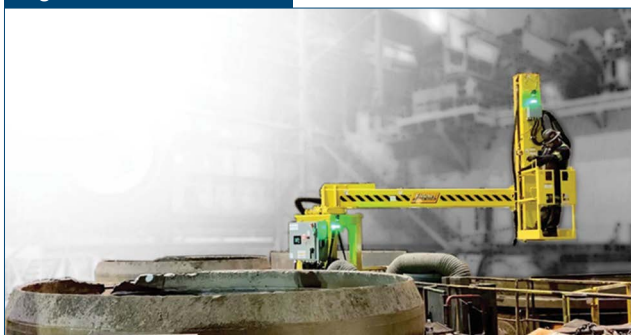
Dual ladle access device (LAD) installation.
