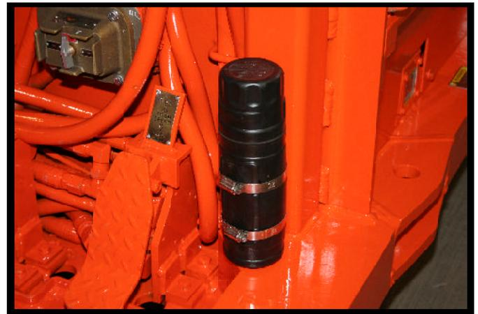
In the past, Fletcher only provided a set of a laminated electrical prints with each new machine when shipped. In response to customer requests, Fletcher now includes a set of laminated electrical AND hydraulic prints with each machine. The prints are stored in a sturdy plastic document tube mounted on the machine so they can be accessed easily by maintenance personnel when needed.
