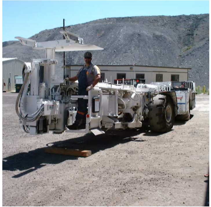
Bolter attached to shield mover
