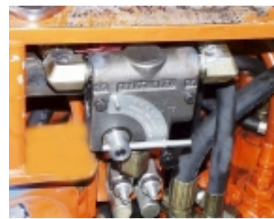
Flow control for adjusting drill speed and impactor frequency
