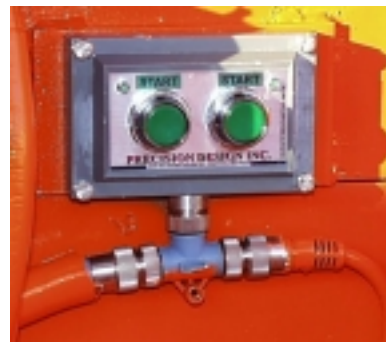
Start Switch In Tram Deck
