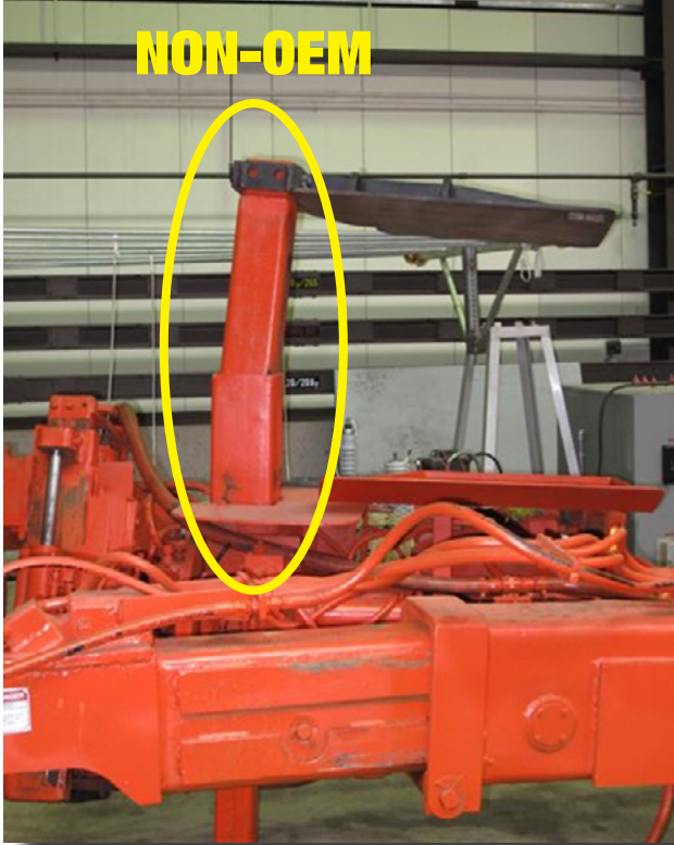
Replacing machine components with Non-OEM parts, such as the leaning canopy support post picture above, voids the Fletcher certification and may not meet required standards.
