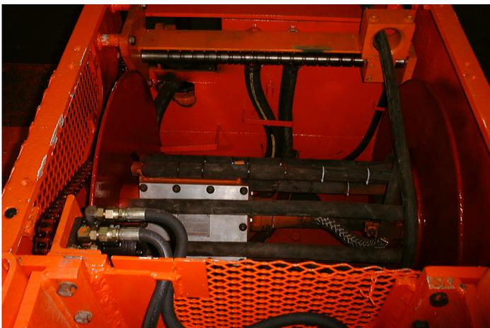
A manual control is provided to allow the machine operator to turn the cable reel ON and OFF as required. The cable reel valve package is located in the circuit to regulate the trailing cable take-up speed and tension. This valve package also contains a relief valve to eliminate cable backlash.
