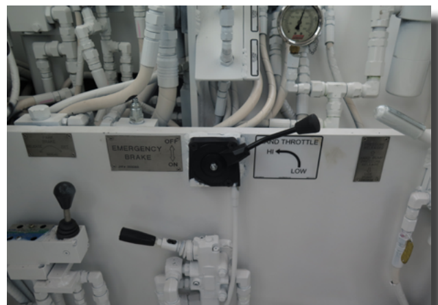
Manual Hydraulic Park Brake and Emergency Brake (Service and Park Brake) Controls
