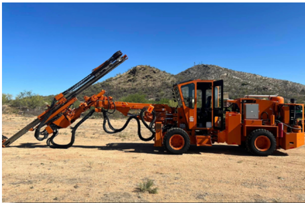
Cannon Single Boom Jumbo Drill, onsite at San Xavier Underground Mine in Arizona.
