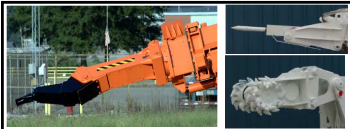
360° Tool rotation with pick or optional hydraulic breaker or cutter drum.
