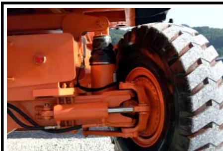
Totally enclosed wet disk brakes on each wheel and nitrogen charged strut suspension
