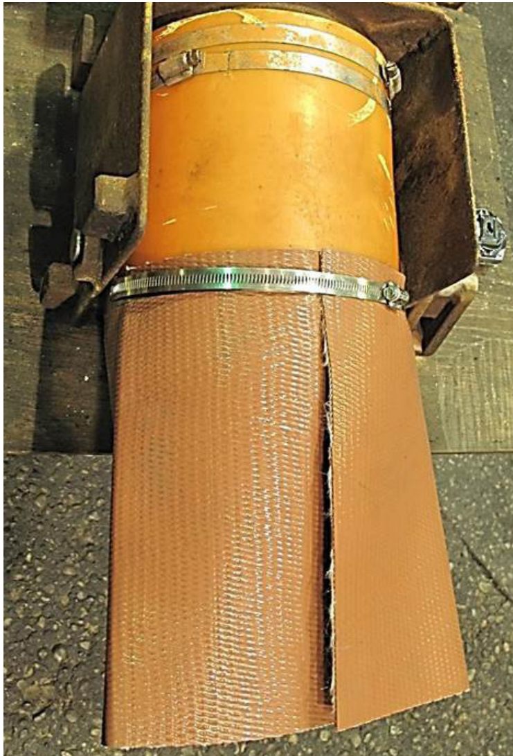
Extension Tube Installed - Ready for Operation in "Dry" Operating Conditions
