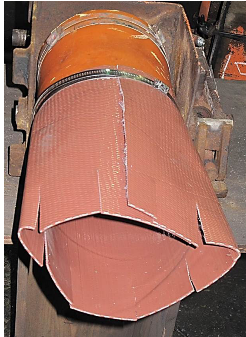
Extension Tube Installed - Ready for Operation in "Wet" Operating Conditions (Slits Cut in Bottom of Extension Tube)
