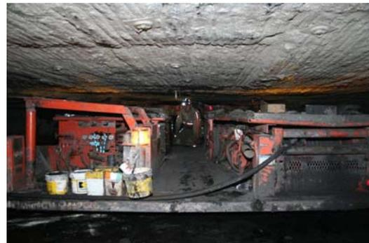
6. Rib access booms were developed on all WT models to allow the operator to better position himself in rib and truss bolt installation.
