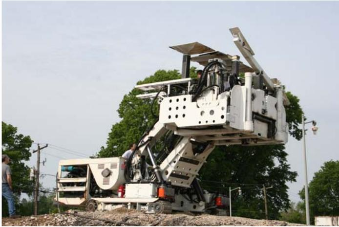
The operator's platform slides out toward the rib. The operators will then start drilling the outside holes making use of detented controls. While that mast is drilling, they can then move to the inside masts and drill those holes.
