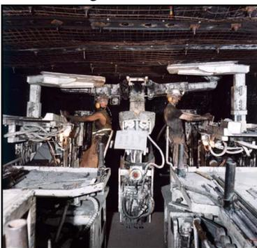
The first model HDDR WT roofbolter was built for Monterey Coal No. 1 Mine in Illinois in the mid 1980's. Soon after, the sales of HDDR WT and other models spread to the Western states and Alabama, and Kentucky.
