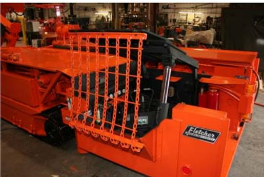
Fletcher has previously introduced the tram deck chain curtain. The chain curtain is mounted from the tram deck canopy. This device
