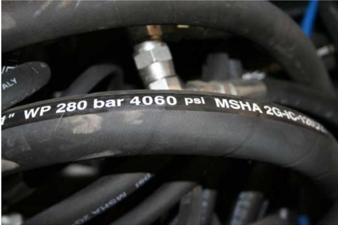
1. An energized circuit has hidden dangers. Always use your company's lock out/tag out program to assure no power is going to the hydraulic power source. Cycle valve handles to divert any pressure to tank (zero pressure). Also, carefully bleed pressure from any line being disconnected
