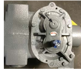
Grease bleed hole in dust shield, above.
