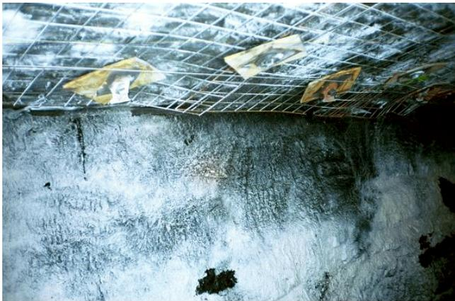
Figure 2. Roof screen achieving up to 94% roof coverage.
