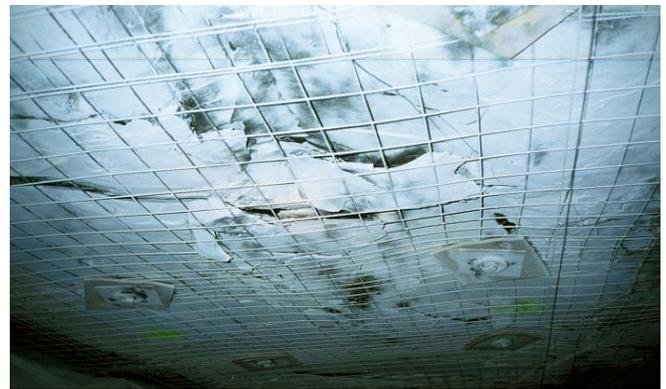
Figure 1. Roof screen effectively controlling weak roof skin.
